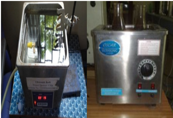
Fig 8: Ultrasonic Cleaner apparatus for sonicator process of AlN & SiC Nanofluids
