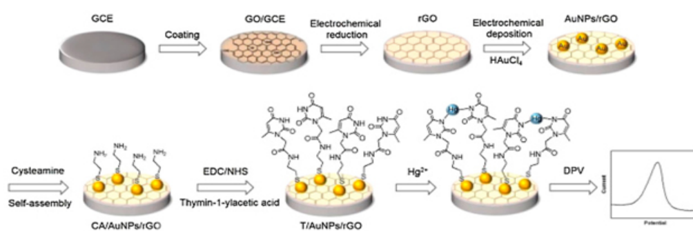
Fig. 2. Scheme of thymidine functionalized biosensor for Hg^{2+} detection. Printed with permission from [25]. Copyright 2016 Elsevier.
